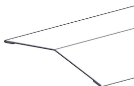
R Wood Roof V Flashing
